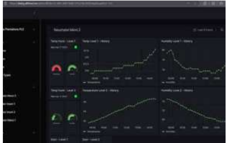
IoT Temperature Monitoring System for Drying Towers
